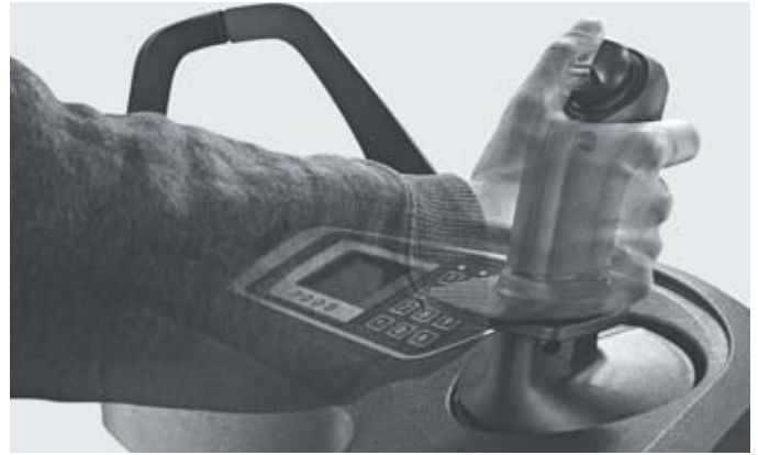
Precise driving, lifting and lowering with standard joystick, without having to keep changing hands for fatigue-free operation
