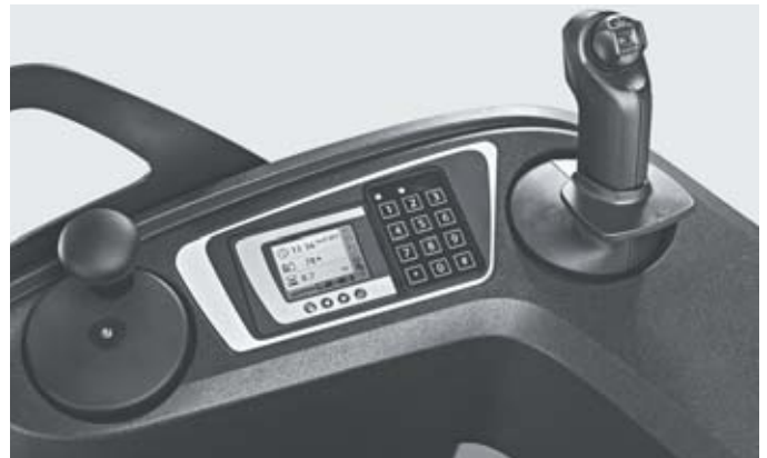
Maximum comfort: The steering wheel can be positioned on the left- or right-hand side for individual adjustments
