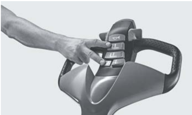
Palpable difference: The control elements can be clearly distinguished because of their tactile characteristics
