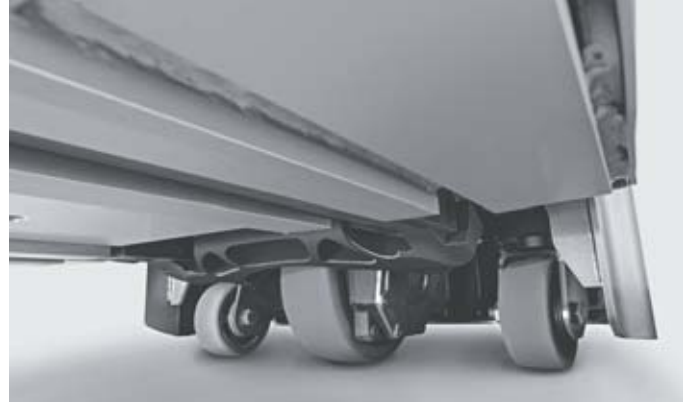
Up the ramp and down again: Traction in any situation due to the hydraulic support wheel suspension
