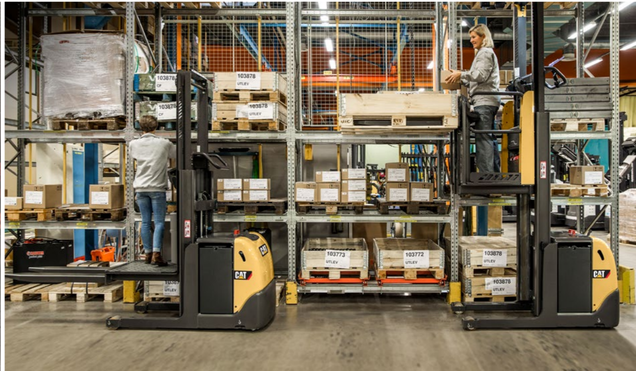
(Pictured clockwise from far left) The NOH12PH is designed for high-level picking at heights up to 12.1 m.
